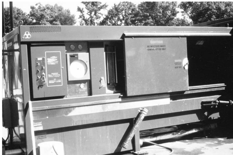
Fig. 8.8 On-site steam autoclave
