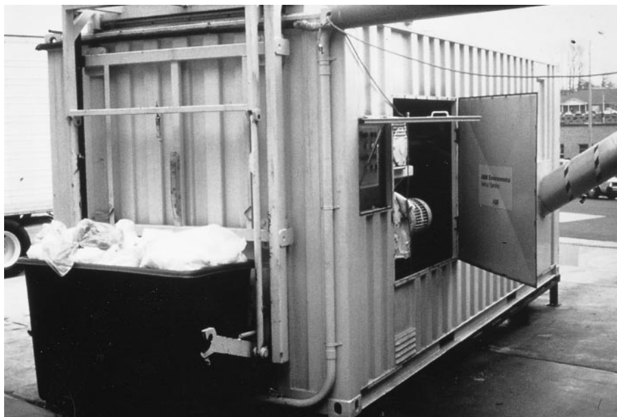
Fig. 8.10 Microwave treatment unit for health-care waste
