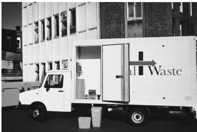
Fig. 7.11 Example of vehicle used for transportation of health-care waste in the United Kingdom
