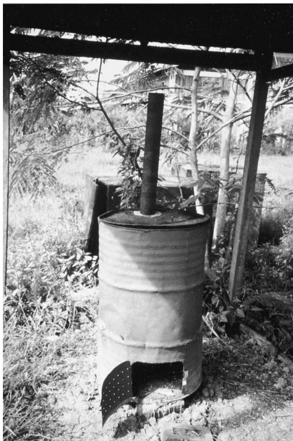
Fig. 8.6 Drum incinerator with chimney
